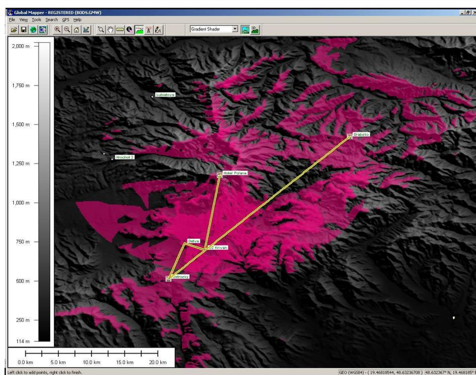
Fig. 4 Location of cameras, data transshipment and direct visibility of cameras [6]
